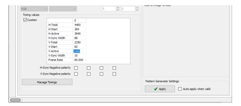
The timing parameters can be modified by selecting the **Custom** check-box and editing the fields of the matrix. Enable the new parameters by clicking **Apply** button.
