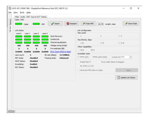
Link tab contains four panels: Cable / HPD, Link Status, Link Configuration and Stream Status.
