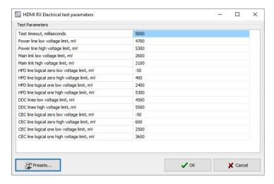
Each test in the Electrical test set uses parameters to control test execution and acceptance criteria. Parameters for all tests are collected in the dialog *Electrical test parameters*.
