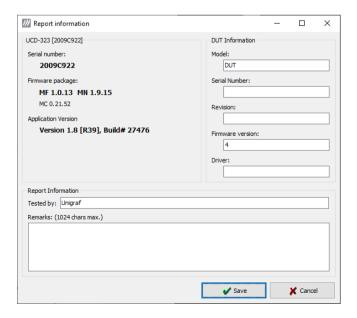
Click **Save Report** in UCD Console. A dialog will open where information about the DUT and remarks about the test can be included in the report. Details of the used test equipment and the software and firmware version will be added automatically.
