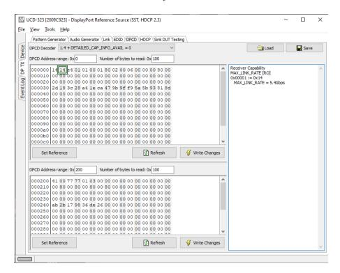
DPCD tab is a tool for monitoring and editing the DPCD registers of the connected Downstream Sink.
