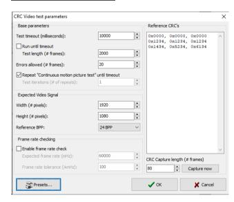
CRC Video test parameters dialog allows you to define the test duration, number of frames captured, and errors allowed. It allows you to define the frame size and capture.
