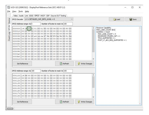
DPCD tab is a tool for monitoring and editing the DPCD registers of the UCD-300 Sink.
