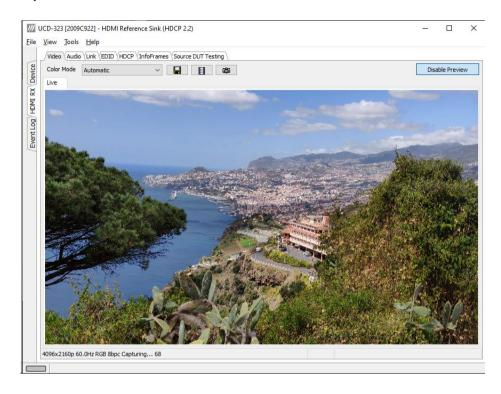
The measured input resolution, frame rate and color format is shown below the preview window. The indication of the number of frames captured to the PC shows you the pace of the image data transfer to the PC.
