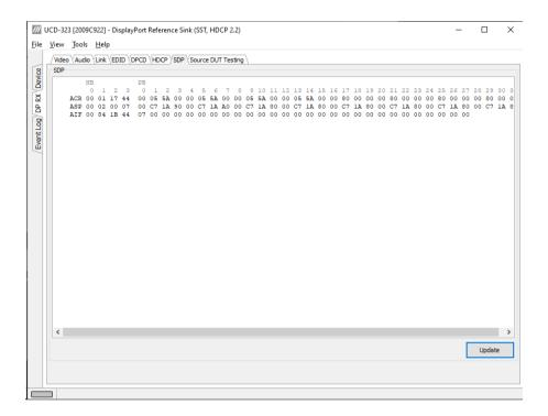
SDP Tab displays in hexadecimal format the following received SDP packets:
