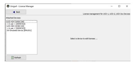
In the list of Attached Devices please select the device in question. You can find the *serial number* and the *seed number* of your device in a sticker attached to the bottom of your device.
