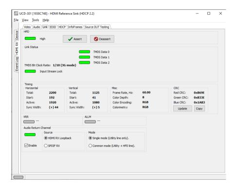
Link tab contains four panels: HPD, Link Status, Timing and Audio Return Channel.
