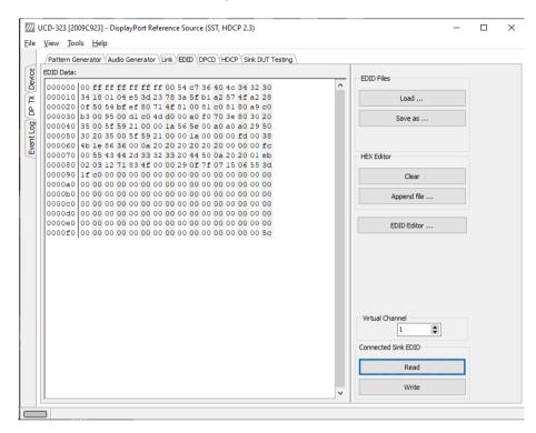
EDID tab will enable analyzing and saving the EDID read from the connected Sink device.
