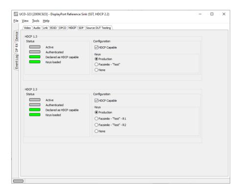
HDCP tab is the dialog for monitoring the HDCP (for *High-Bandwith Digital Content Protection*) status and controlling the HDCP capabilities of the connected UCD-300 device.
