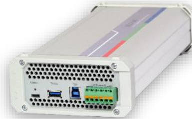
UCD-340 USB Type-C DP Alt Mode tester
