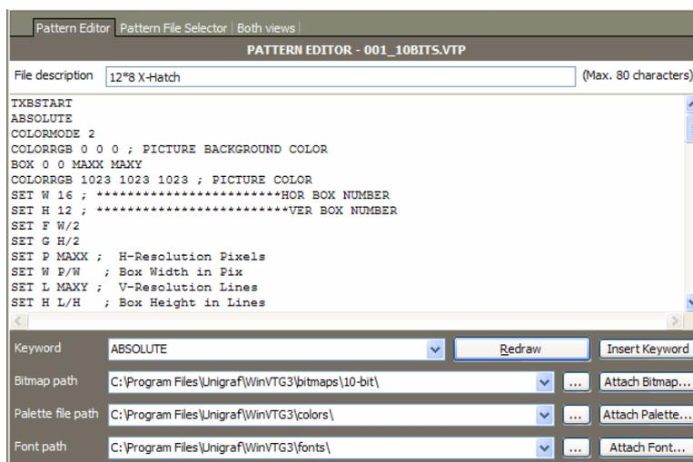
After editing the pattern definition click **Redraw** or press <F4> for updating the displayed pattern. The VTP language keywords with their parameters can be selected from the pull-down menu in *Keyword* field. Select one of the commands and click **Insert Keyword**.
