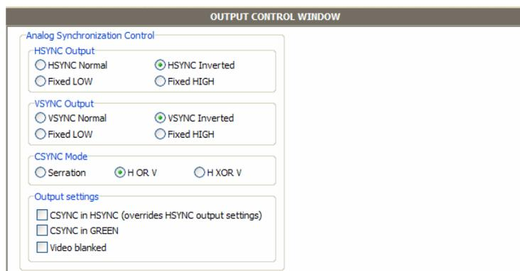
You can set the Horizontal sync options from the **HSYNC Output** panel, the Vertical sync options from the **VSYNC Output** panel and the Composite sync mode from the **CSYNC Mode** panel. From the **Output settings** panel you can define where the composite sync appears. When **Video blanked** option is selected, no syncs are present in the output.
