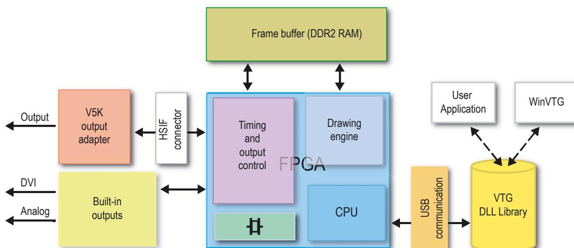
VTG-5225 design is based on an advanced high speed FPGA. The FPGA consist the program execution unit *CPU*, the *Drawing engine* and the *Timing and output control*. The test patterns are stored in the *Frame Buffer* and clocked out to *Built-in outputs* or *V5K output adapters* via the *HSIF connector*.
