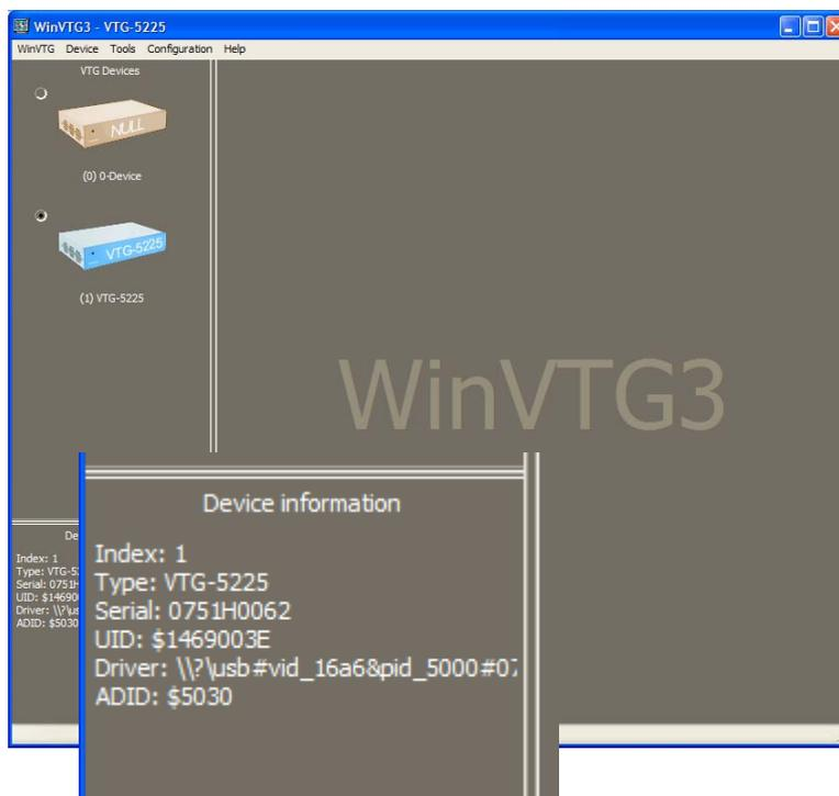
The *Device Information* lists the type designation, the serial number, and ADID, the identification of the V5K output adapter if one is present.
