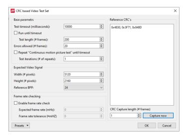
TE compares the video mode (Frame Width, Height, BPP and optionally Frame rate) to provided parameters and after that captures frames and compares the CRC (check sum) of their three color components to the provided reference until the number of bad frame limit provided is detected or the provided total number of frames is reached.
