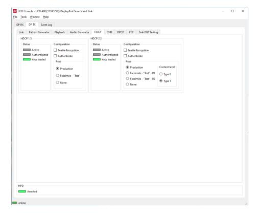
HDCP tab is the dialog for monitoring the HDCP (for *High-Bandwith Digital Content Protection*) status and controlling the HDCP capabilities of the UCD device.
