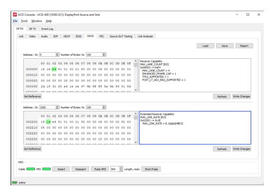
The *DPCD Decoder* panels on the right show the interpretation of the DPCD byte selected on the monitoring windows. The selected byte is shown with a green background.
