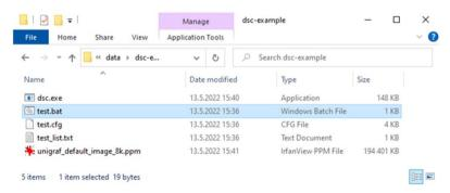
In the example, the DSC conversion is done using batch file *test.bat*. It is creating DSC content from *unigraf\_default\_image\_8k.ppm* using VESA created tool *dsc.exe* and its parameter file *test.cfg*.
