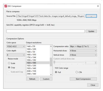
Select the source bitmap file in Source File field. Define the Output Resolution, the color depth, compression ratio and number of horizontal and vertical slices in the frame.
