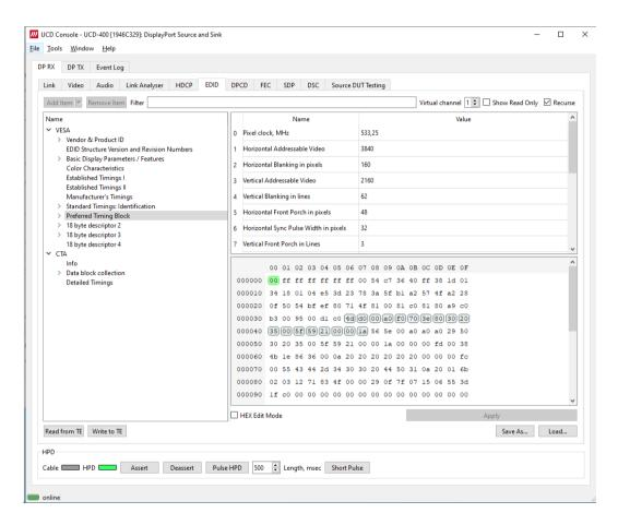
The EDID Editor main window is divided into three logical areas. The bottom part additionally contains the command buttons. The top-left portion shows the currently edited E-EDID blocks in a tree-form, and the top-right portion shows an edit control for the currently selected item, possibly a list of sub-keys and their names (The list is not shown for all values) and the HEX-view of the block collection.
