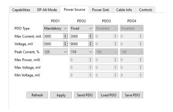
PDO Type: Definition of power source type (Disabled, Fixed, Variable or Battery)
