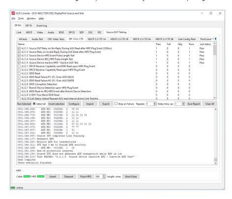
At the completion of each test the result of the test is indicated in the matrix on the right hand side of the test panel. For each test the matrix lists the number of occurrences of each result and the number of tries performed.
