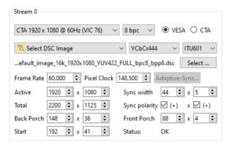
When a DSC image is selected as the pattern, UCD Console will automatically enable DSC, provided that the connected Sink device declares support for DSC in its DPCD.
