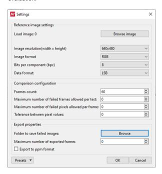
The test compares the captured frames to a provided reference image on pixel level.
