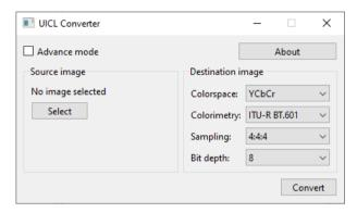
Image Converter has two operating modes: Standard mode and Advanced mode. In Standard mode typical Windows image file formats are used as Source image and the user sets basic color formats for the Destination image. In Advanced mode, the user is able to define the Source and Destination image parameters in detail.
