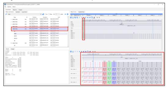
The image below further shows you how the different areas of the TimeLine Viewer align when you double click on a frame in *Wave Form View*.
