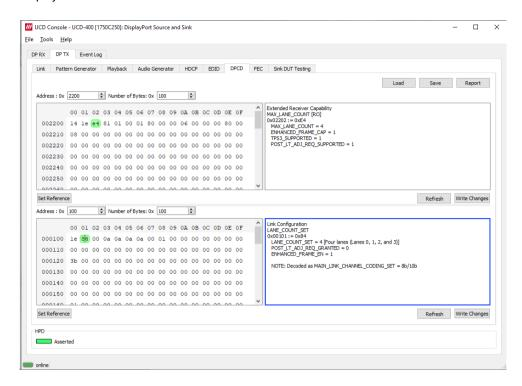
The *DPCD Decoder* panels on the right show the interpretation of the DPCD byte selected on the monitoring windows. The selected byte is shown with a green background.
