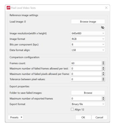
The test compares the captured frames to a provided reference image on pixel level.
