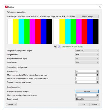
When the preview has been enabled click the *Capture reference* icon to store a frame and use it as reference. Before accepting the frame, stability of the video is verified with a CRC stability check. Captured CRC can also be verified by the user.
