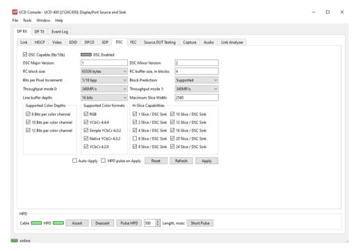
Enabling DSC feature is controlled by the connected source device. When connected, a source verifies corresponding registers in DPCD of UCD sink to find out if DSC capability is declared.
