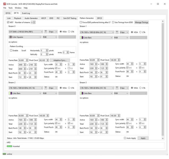
MST: Checkbox for enabling Multi-stream transport (MST) mode. (UCD-400, UCD-411, UCD-424 and UCD-451)
