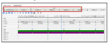
When you zoom in more, the frames shown in *Wave Form View*, are highlighted in green in the scroll bar as shown in the image below.
