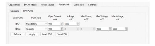
PDO Type: Definition of power source type (Disabled, Fixed, Variable or Battery)
