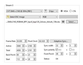
When a DSC image is selected as the pattern, UCD Console will automatically enable DSC, provided that the connected Sink device declares support for DSC in its DPCD.
